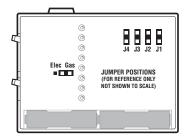
There are five options which are set by jumpers on the rear of the units circuit board. Four are set by A GROUP OF numbered jumpers. They are:
