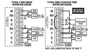
C A U T I O N Do not allow wires to touch each other or parts on thermostat. Terminated wires must be trapped between black spacer and brass terminal. Securely tighten all 8 electrical terminal screws.
