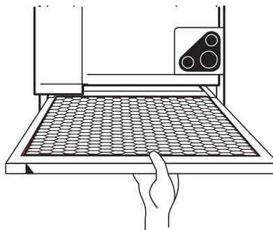
Slide dirty filter out, replace with a new filter making sure the arrows printed on it are pointing in the direction of airflow. Hold the "FILTER" door firmly in place and snap the levers down (closed).
