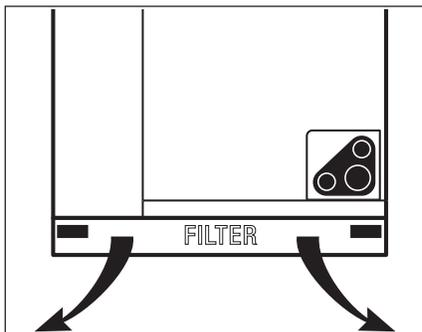
Locate access door marked "FILTER" and lift up the open side of the levers.
