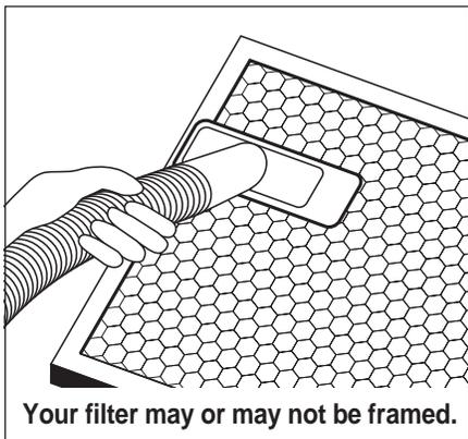
must be replaced every month with the same size as originally supplied. Both methods are quick and easy and guaranteed to cut the energy used by your system. When replacing your air handler filters,
