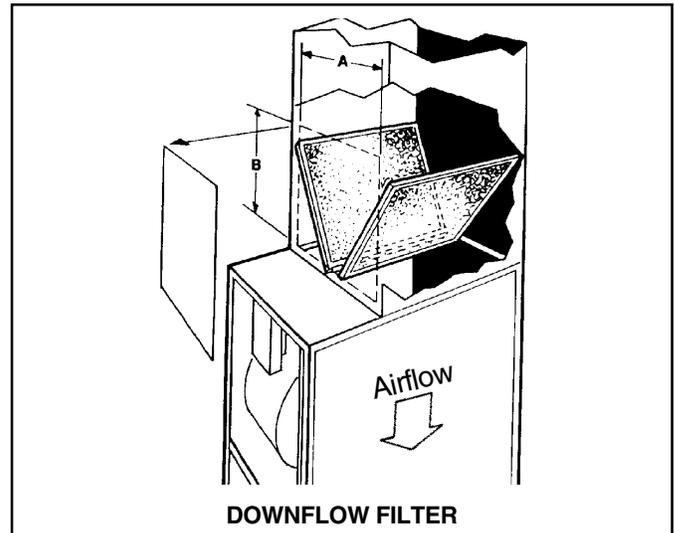
A downflow/horizontal furnace return air filter application, as shown, features two 14" x 20" x 1" filters in the 17-1/2" wide furnace cabinets; or two 16" x 20" x 1" filters in the 21" and 24-1/2" wide furnace cabinets.
