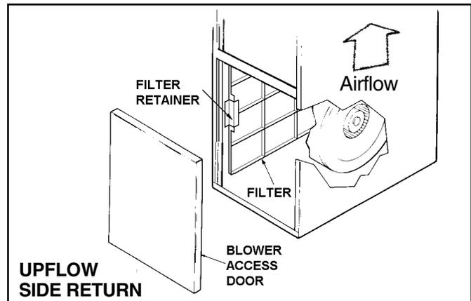
For vertical UPFLOW ONLY, a left or right return air inlet as above (left side shown) requires trimming of the factory supplied filter to 17" x 25" x 1" for both the 21" and 24-1/2" wide furnaces.
